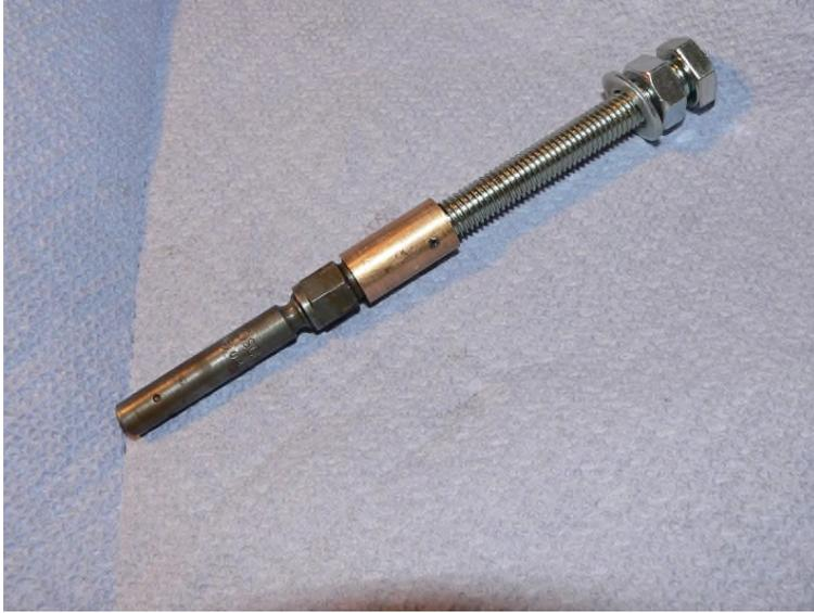
Pressing injector into a seal:
